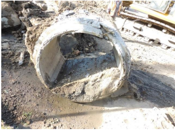
Storm Main Renewal 6 th Ave W – Pipe in poor condition with reduced capacity.
