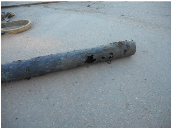
Sample of Corroded Valve Boxes.
